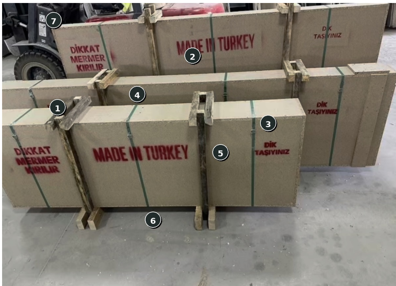
Supplied workshop photo showing completed protected assemblies, orientation markings, timber restraint and nearby forklift handling context.
